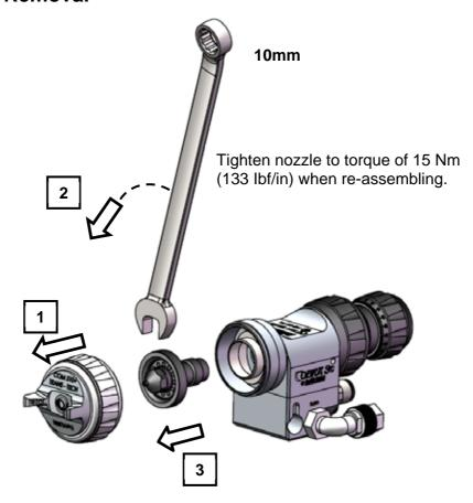
**Manifold O-Ring and Connector Removal/Assembly**
