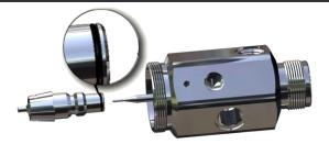
5. Withdraw liquid insert [20] by hand. Check the O-Ring [21] of the liquid insert for any damages and replace it, if necessary.
